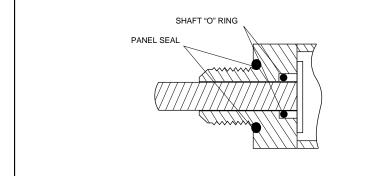
The shaft is sealed by an O-ring inside the bushing. The panel is sealed by an O-ring at the base of the bushing.
