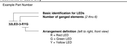
Example part number describes a stack of 3 LEDs, arranged red, yellow and green from left to right. Maximum number of stacked LEDs in this part numbering scheme is six. Contact Grayhill for stacks of more than six elements.
