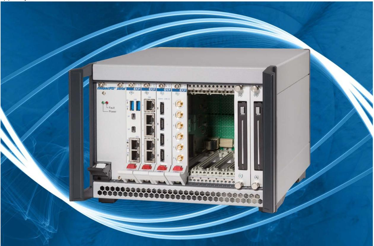
**SC2-PRESTO • CompactPCI® Serial CPU Board • 4<sup>th</sup> Generation Intel® Core™ Processor**
